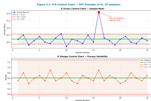
Figure 2.2: \bar{X} -R Control Chart — Sample Mean and Range Chart showing Out-of-Control signal at sample 16
